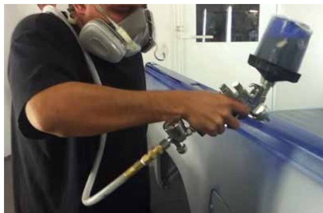
Figure 2: Spray-painting work with isocyanates (low molecular weight chemicals)
