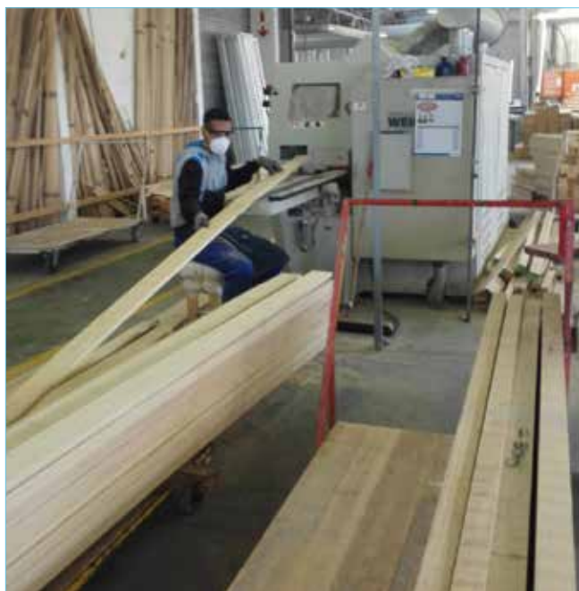
Figure 2d: Wood-planing and thicknessing section
